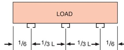
**Stacking Height and Vertical Arm Spacing**
